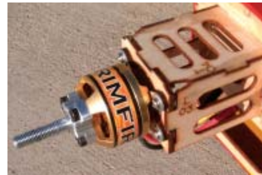
The ply motor mount is well designed and can be easily mated to many of a range of inrunner or outrunner motors.
