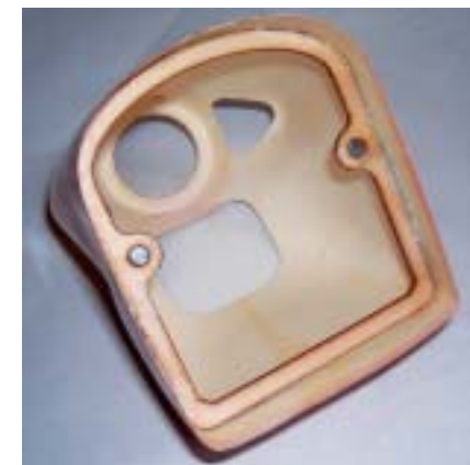
Note the magnets glued into recessed holes in the cowl. This system worked well.
